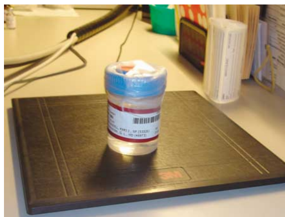
Figure 1. Specimen bottle with a MERGE database-generated label and RFID tag (on the bottom of the bottle) on RFID pad. RFID, radiofrequency identification.
